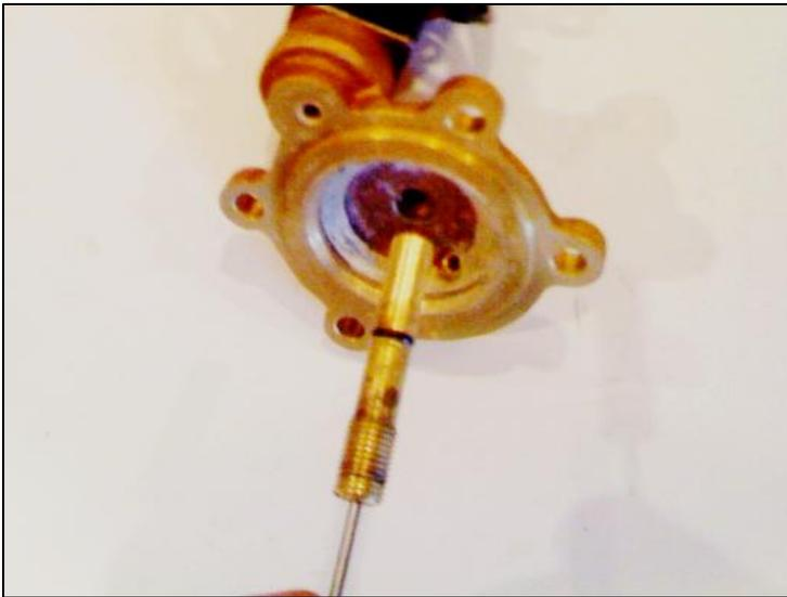
**PROBLEM:** Water leaks out between adaptor and anti-siphon body.
