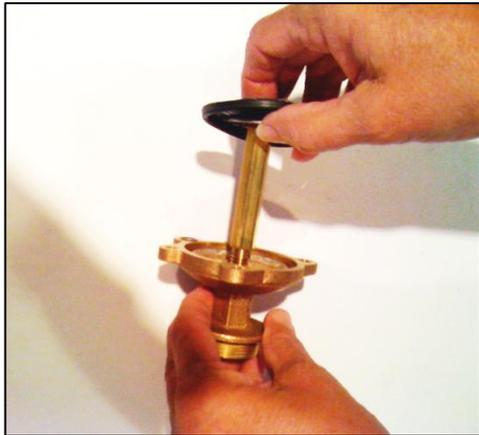
6. To disassemble diaphragm assembly, use a 7/16" wrench to hold shaft, and 9/16" wrench to remove nut at top of diaphragm shaft.
