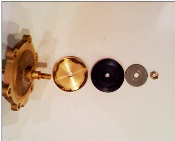
**PROBLEM:** Valve will not close and water constantly exhausts from vent hole in chamber-plate (located on rear side of valve).
