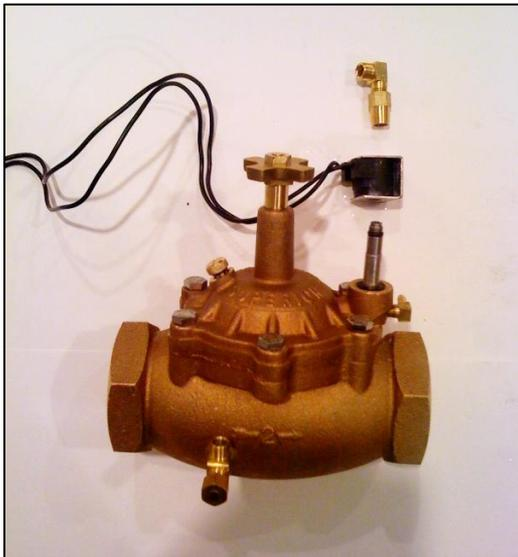
4. Using a flathead screwdriver, unscrew solenoid post from bonnet.
