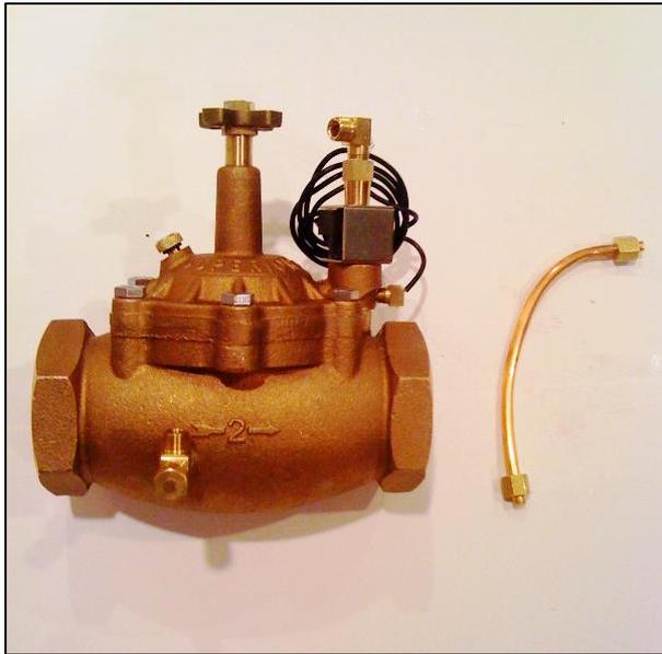
2. Apply ½” wrench to hex portion of coupling that connects solenoid post to L-fitting and unscrew coupling and L-fitting from solenoid post. It is not necessary to separate L-fitting from coupling.
