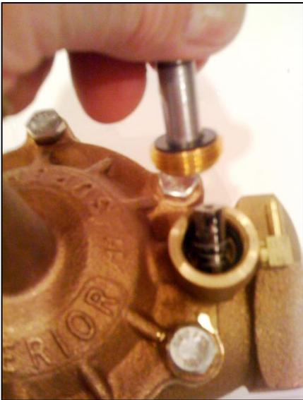
6. The photo shows the solenoid cavity of the model 3300. The port directly to the right of the exhaust port (center port) serves no function. The port directly above the exhaust port in this photo leads to the lower diaphragm chamber. The exhaust port leads to the barbed L-fitting where water in lower diaphragm chamber exhausts to atmosphere when solenoid is energized.
