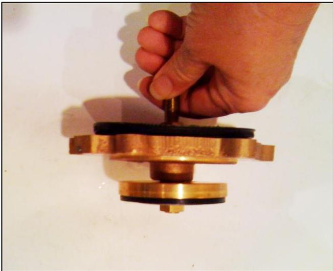
**PROBLEM:** Valve will not close when energized and water exhausts continuously from the barbed L-fitting (but stops when solenoid is de-energized).
