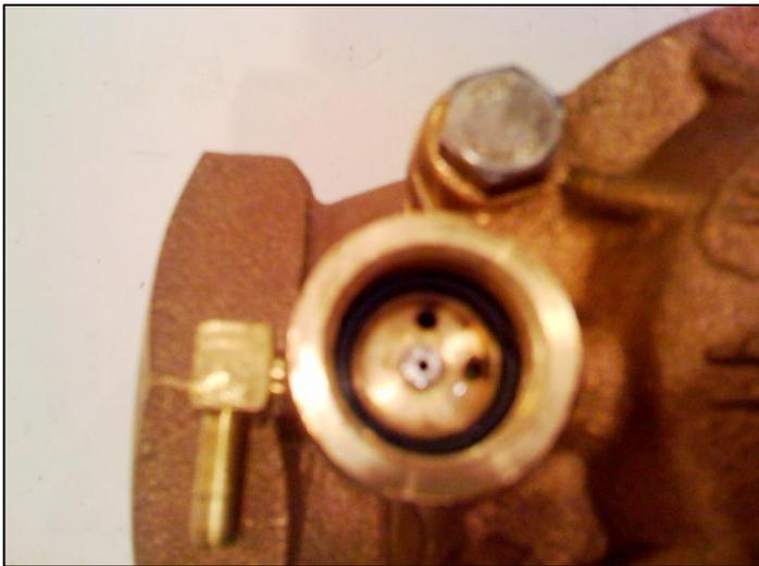
**PROBLEM:** Valve does not fully open when solenoid is not energized.
