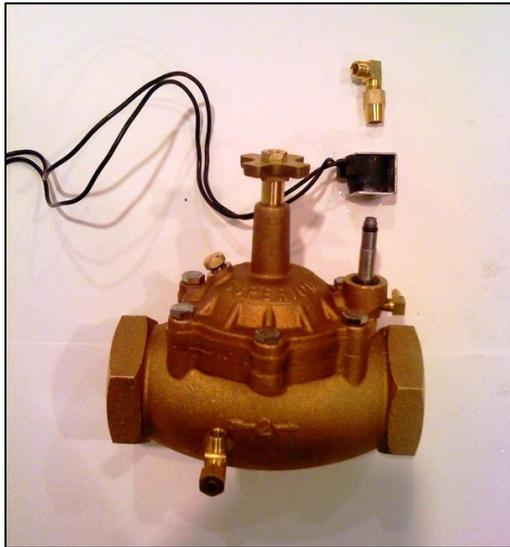
4. Using a flathead screwdriver, unscrew solenoid post from valve bonnet.
